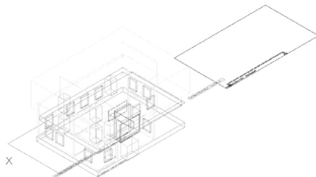
**Proxygraphics = 0;** Does not save the geometry of the objects in the drawing. Vanilla ACAD will display objects as bounding rectangles with a descriptor box telling you this is an AEC object.
